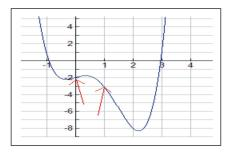
We can see that the graph has two relative minimums, one relative maximum, and two inflection points (as indicated by arrows).
