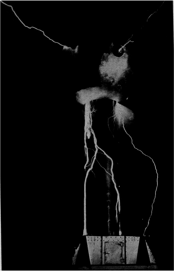
PLATE IV. Sparks in the Van de Graff electrostatic generator. The man-sized door at the bottom gives some idea of the height of the structure. (See p. 77.)
