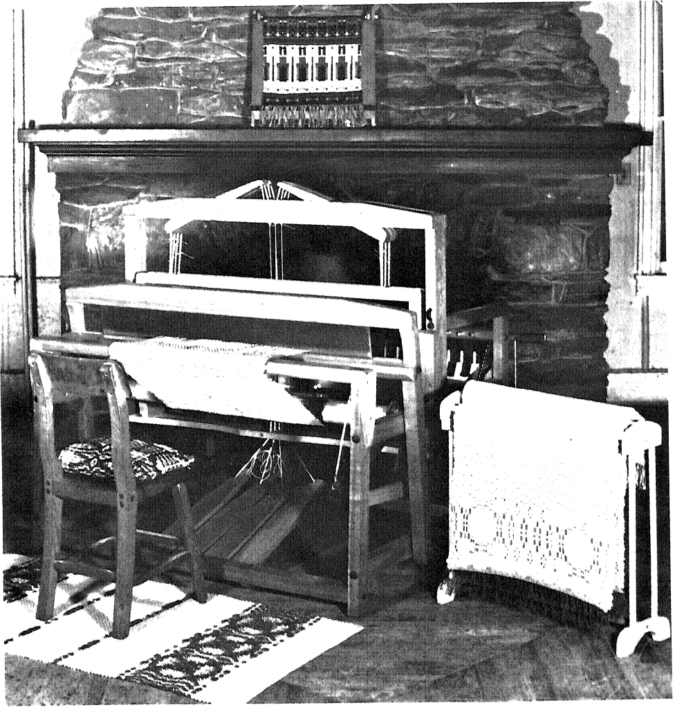
Fig. 6 — A rug loom and its products. The loom is a 4-harness jack type.
