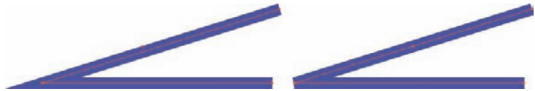
FIGURE 6.13 A sharp corner results in a long spike in the stroke (left), and a miter limit clips the stroke (right).
